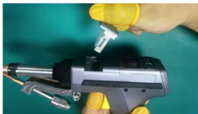
② Remove the protective lens holder
