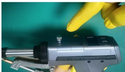
① Unscrew the protective lens screw
